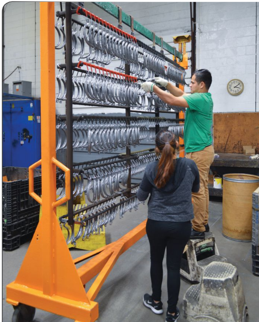
The shop also offers services such as powder coating, hydrogen embrittlement baking, ultrasonic cleaning, acid pickle and oil, polishing, vibratory and part deburring.
